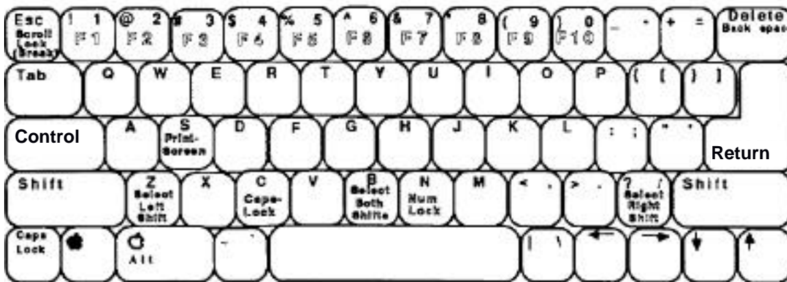
Apple II gs Keyboard to IBM Style Keyboard Translation
